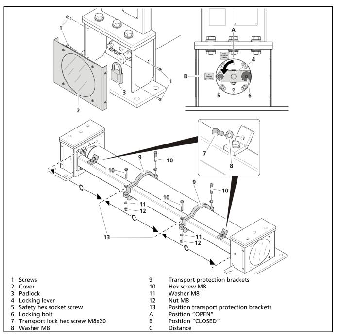
Close radiation beam outlet and mount transport brackets
