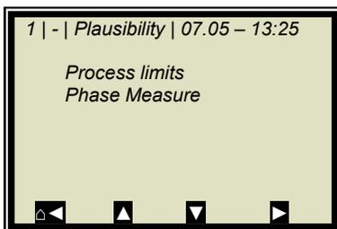
The **process limits** need to be adjusted. Allow exceeding of the measuring by  $\pm 5\%$  absolute. Example: The measuring range is 65-95% TS. Enter 60-100% TS as process limit.
