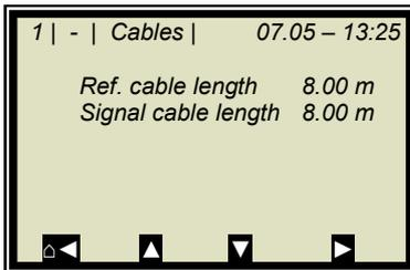
If the factory-set cable lengths do not match the actual geometry conditions, you have to correct the values.
