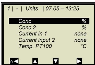
The units of the concentrations (conc 1 and 2) and those of the enabled analog inputs can be selected.
