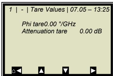
Enter the last recorded values of Phi(fm) and attenuation, taking into account the algebraic sign "-".
