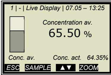
Push **ESC** to go to the main menu. A measurement can be stopped only in the main menu.
