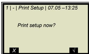
Push the  button to print the setup via RS232 and RS485. Push  to go back one page without printout.
