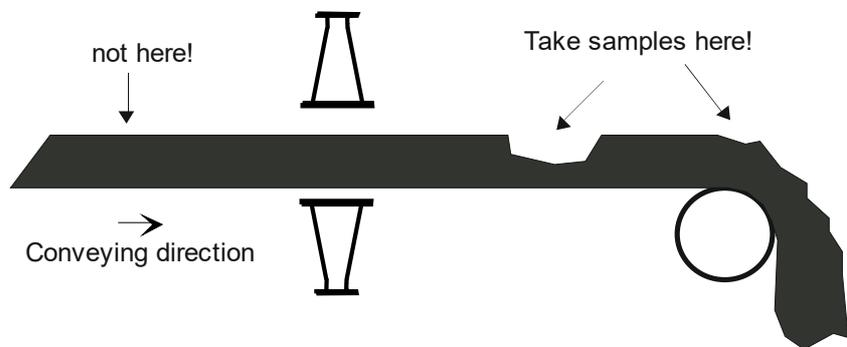
Figure 7-1: Sampling point on the conveyor belt
