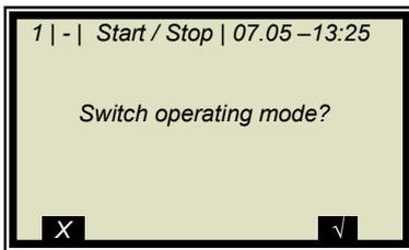
Push **✓** to confirm the prompt and the measurement switches to the **STOP** mode.
