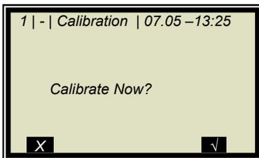
Push the **✓** button to start the calibration; push **X** to go back one page without calibration.
