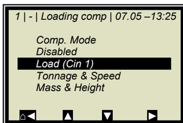
In the case of compensation of the material layer thickness, e.g. with the ultrasonic sensor, select:
