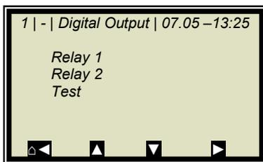
The meter has two relays. Relay 1 is linked with LED signal 1 and relay 2 with LED signal 2.
