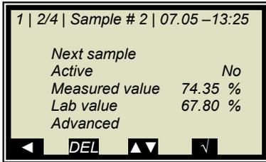
Make sure that all samples have been processed and only those samples are active which are relevant for this calibration.
