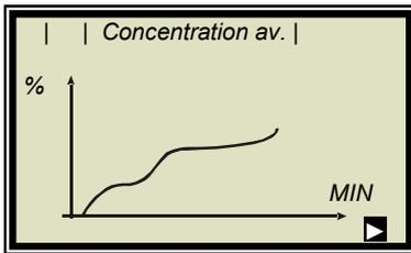
By pushing the **ZOOM** button for a longer time, the enlarged measurement value will be displayed as trend over the entire display.
