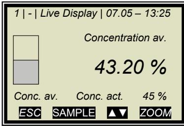
Push the **ZOOM** button to enlarge the measurement value which is surrounded by a frame.
