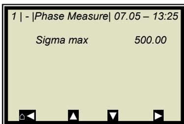
In the normal measurement mode **Sigma** is between 0 and 500. Therefore,  $\text{Sigma}_{\text{max}} = 500$  is a good choice for most applications. Higher Sigma values usually indicate a fault, such as continuous air bubbles which have to be eliminated.
