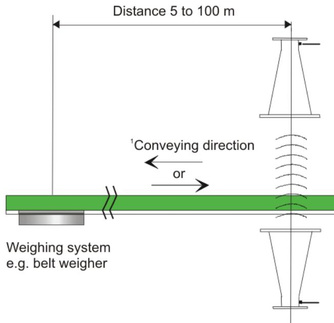
**Belt speed** The belt speed should not exceed 5 m/s when the synchronization is used.
