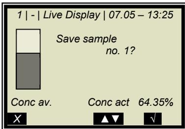
If the sampling process has been completed without any problem, push the  button to save the sample in the table and the measurement continues.
