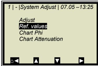
Starting from the main menu, go to the display shown on the left via | SETUP | CALIBRATION | SYSTEM ADJUST |
