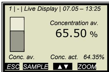
The display reading is now compared with the analysis value of the lab sample. The difference has to be entered as offset with the correct algebraic sign.
