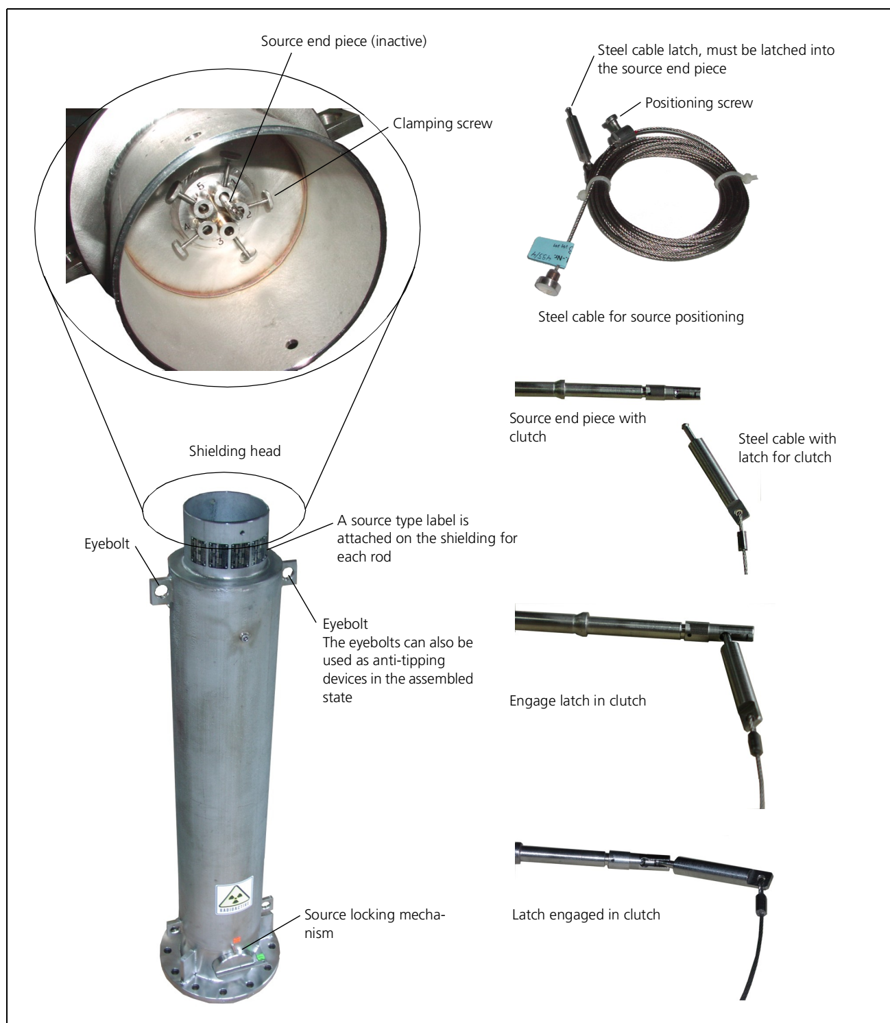
Fig. 2-32 Flange shielding with steel cable
