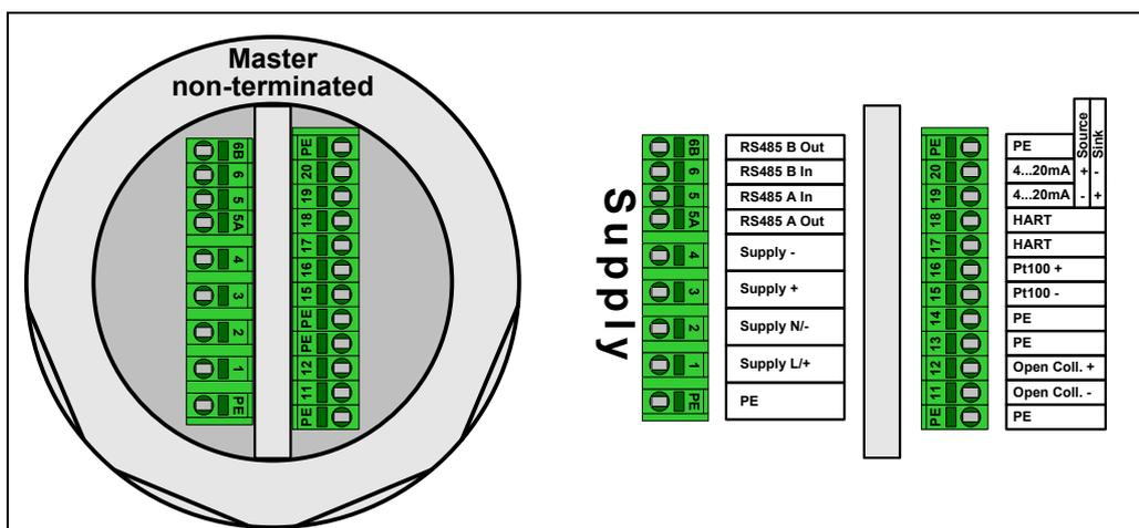
Fig. 7 Terminal Compartment Ex-e and XP (RS485 non-terminated)
