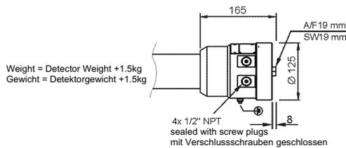
The detector version for divisions (NEC/CEC) differs only in the terminal housing, compared to the standard version illustrated above. The dimensions of this terminal housing are illustrated in this drawing.
