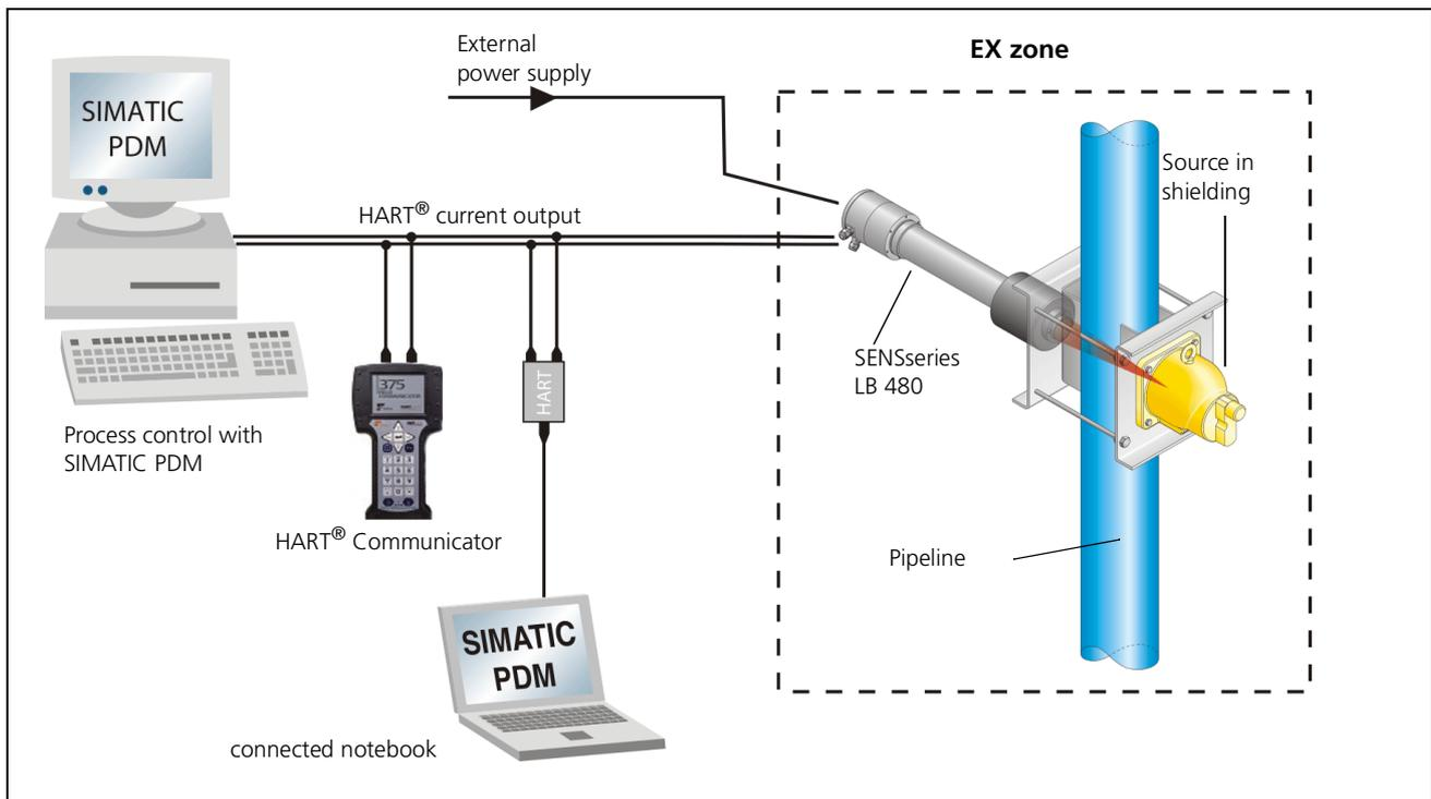
Fig. 1-1 Basic measuring configuration
