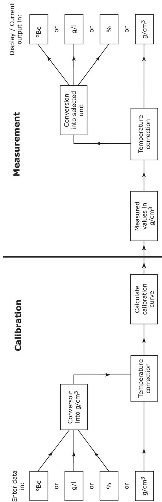
Fig. 7-3 Calculation of suspensions
