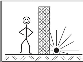
The material surrounding the source provides the shielding effect. As the shielding effect depends, following an exponential function, on the product of thickness multiplied by the density, it follows that materials with a high specific weight are to be used for shielding purposes. The device designer usually calculates suitable dimensions.
