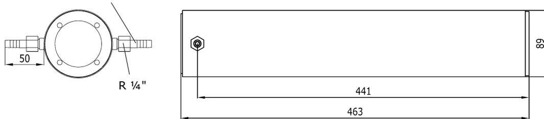
Fitting adaptor for standard water cooling Rp 1/4" → 1/2" NPT
