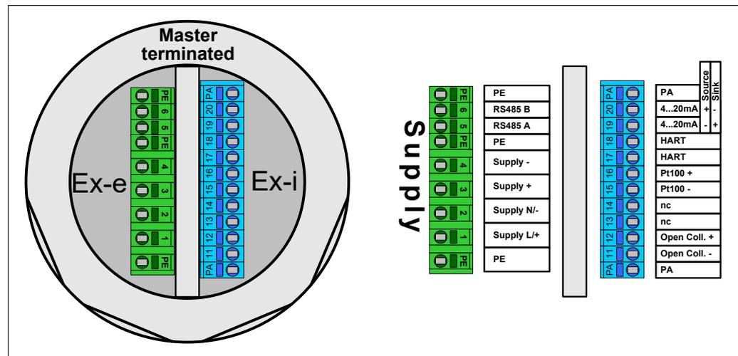
Fig. 8 Terminal compartment Ex-e / Ex-i (terminated)
