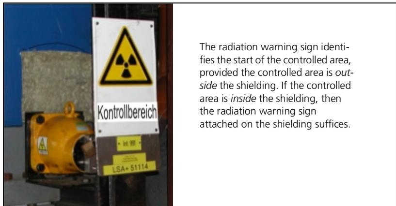
The radiation warning sign identifies the start of the controlled area, provided the controlled area is *outside* the shielding. If the controlled area is *inside* the shielding, then the radiation warning sign attached on the shielding suffices.
