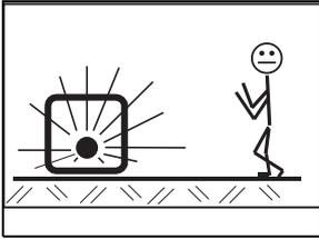
This means the distance between the radioactive source and the human body. The radiation intensity (dose rate) decreases – like light – in proportion to the square of the distance, i.e. doubling the distance to the source reduces the dose rate to one quarter.
