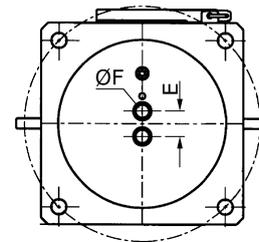
Junction Box for Shaft Core or Steel Cable
