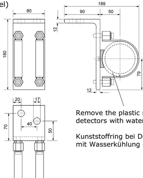
Remove the plastic ring for detectors with water cooling.
