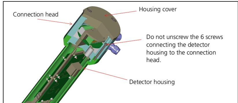
Fig. 3-3 Detector housing with connection head
