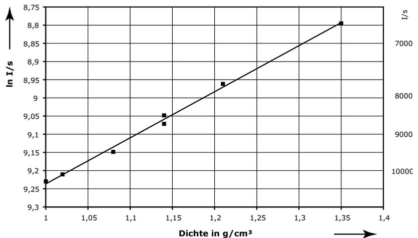
Fig. 5-1 Example of a multi-point calibration
