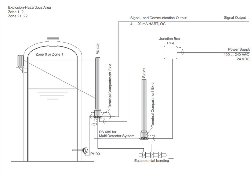
Fig. 5 Installation plan type of protection
