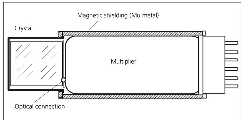
Fig. 4-4 Crystal-multiplier assembly
