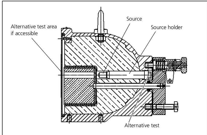
*Fig. 9-2 Alternative test area on point source shieldings:*
