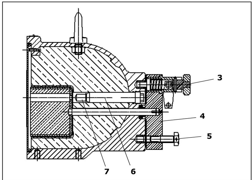
Fig. 10-2 Sectional drawing of source holder, beam path open
