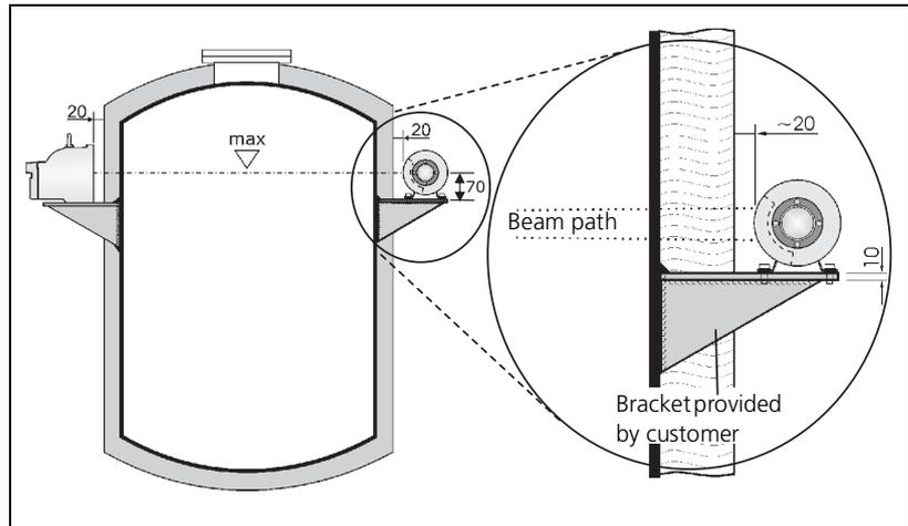
Fig. 2-6 Installing the CrystalSENS
