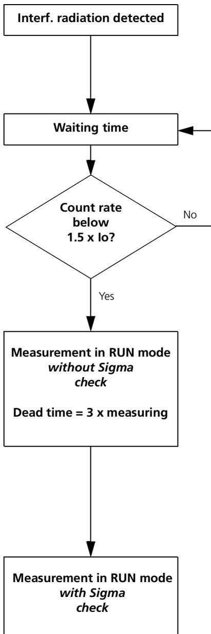
If the count rate is below 1.5-times the empty count rate, the measurement automatically switches to the RUN mode. Sigma detection (see scenario B) is disabled for 3 x measuring time (= dead time).
