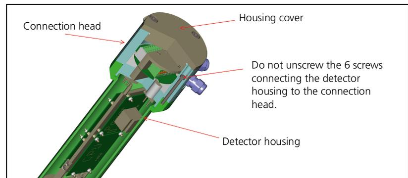
Fig. 1-3 Detector housing with connection head
