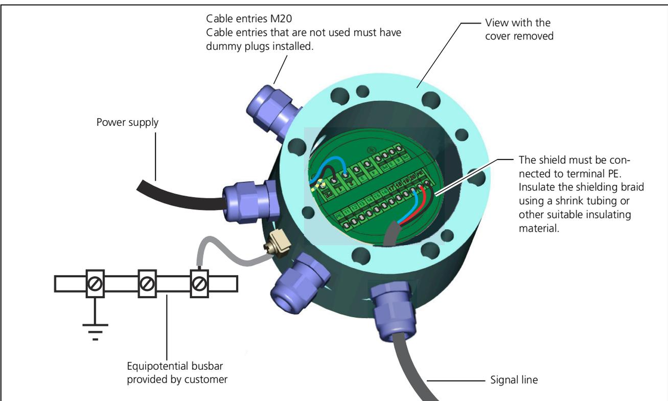
Fig. 3-1 Detector housing open - top view
