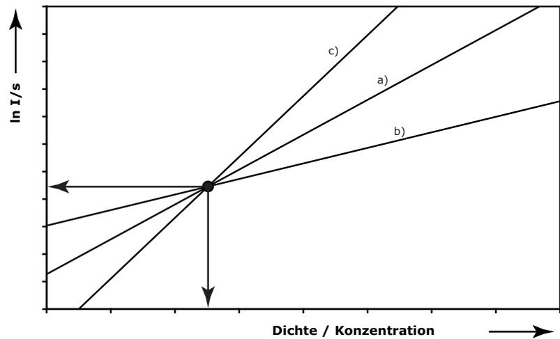
*Fig. 5-2* Influence of the absorption coefficient
