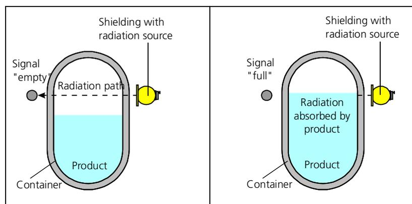
The "Empty" signal is displayed on the analog current output with 4 mA, the "Full" signal with 20mA.
