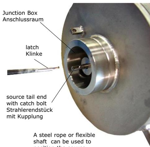
A steel rope or flexible shaft can be used to position the source.
