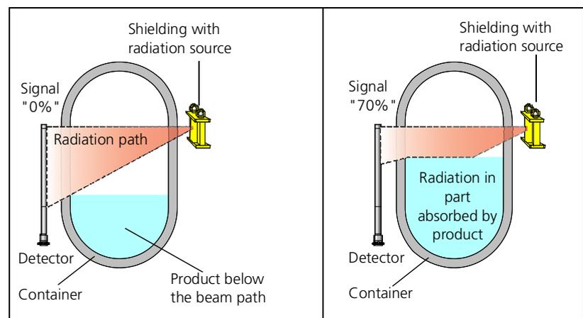
The level change from 0 ... 100% is represented by the analog current output 4 ... 20mA.
