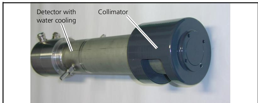
*Fig. 2-12 Detector with water cooling and collimator*
