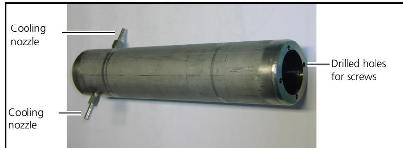
Fig. 2-8 Water cooling
