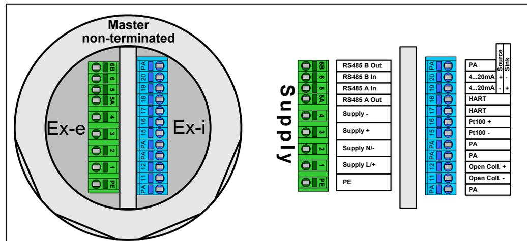
Fig. 9 Terminal compartment Ex-e / Ex-i (not-terminated)
