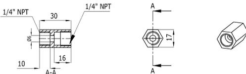
Further fitting adaptors for standard water cooling jacket:
