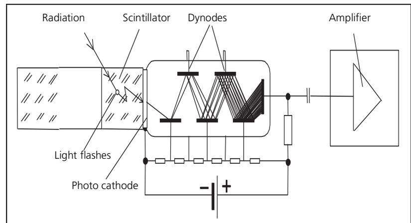
Fig. 4-2 Scintillation detector
