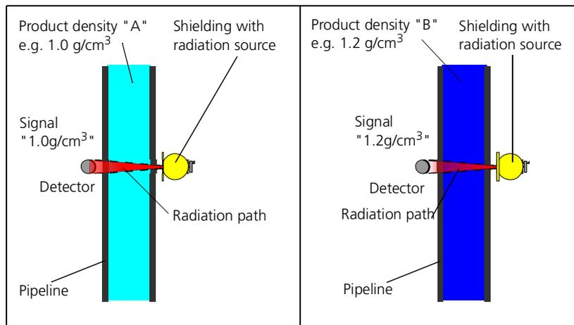
The detector signals the change in density via the analog current signal. The lower measuring range of the density corresponds to 4mA, the upper range corresponds to 20mA. The PT100 may be used for temperature compensation.
