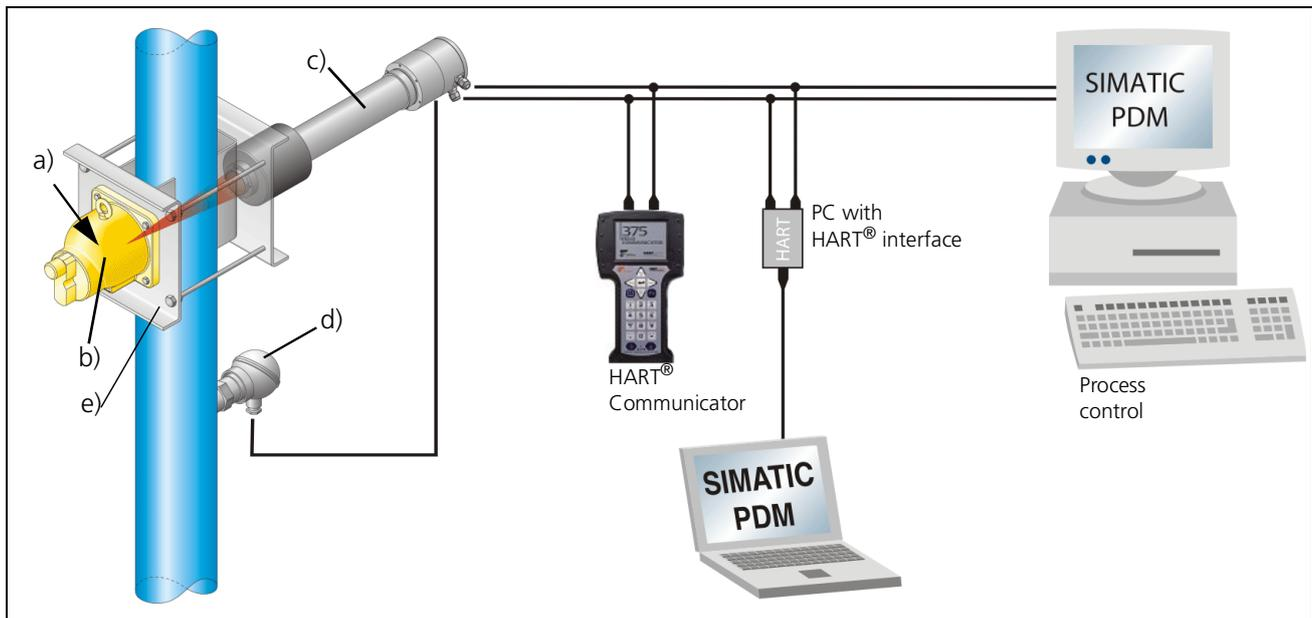
Fig. 1-5 Point source / Point detector arrangement
