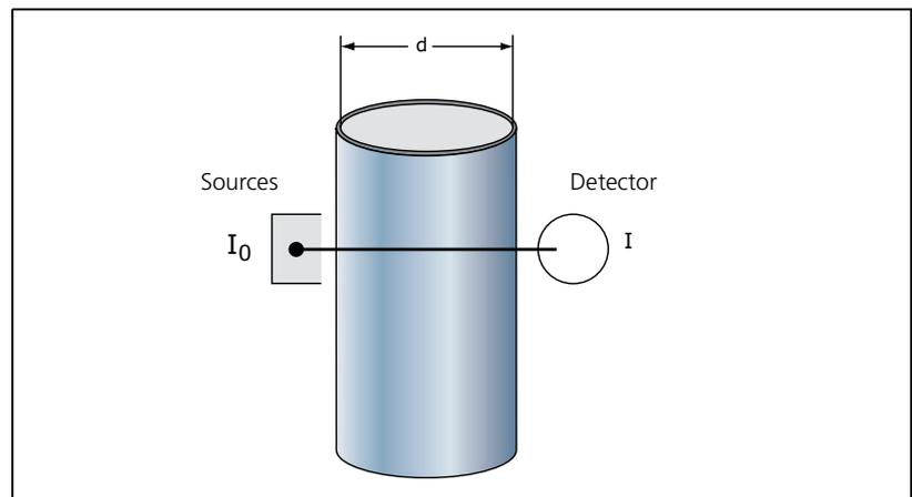
Fig. 1-4 Measuring Principle
