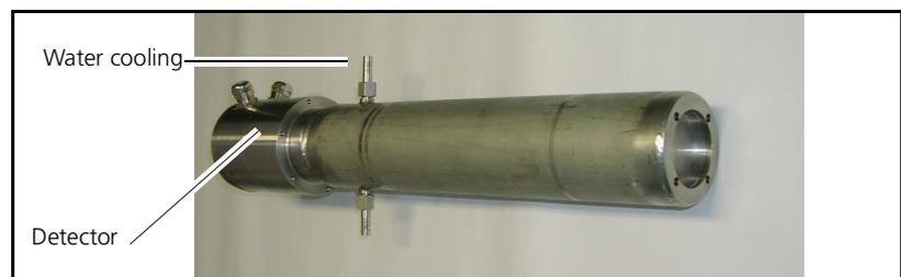
Fig. 2-10 Detector with water cooling
