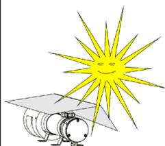
Direct sun radiation can overheat the detector. If the detector temperature can reach more than 50°C, a suitable sun roof must be installed. The heating of the detector by thermal radiation from the vessel can also be moderated by a thermal sheet, e.g. by a thin metal plate. For each detector a water cooling (option) is available.
