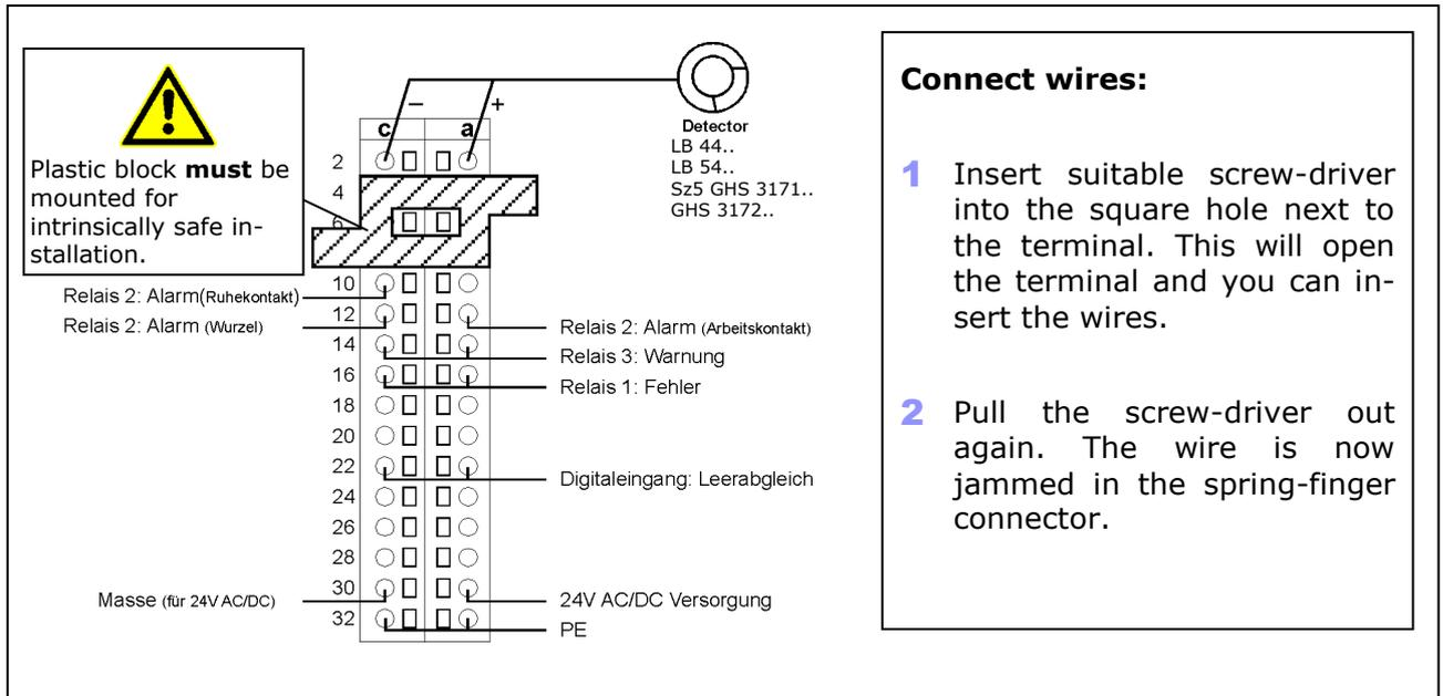
Figure 56: Pin assignment of terminal block
