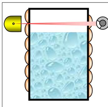
Cooling or heating jackets have to be filled for calibration. In order to preserve the density of the cooling/heating liquid, it should have the same temperature as under operating conditions.
