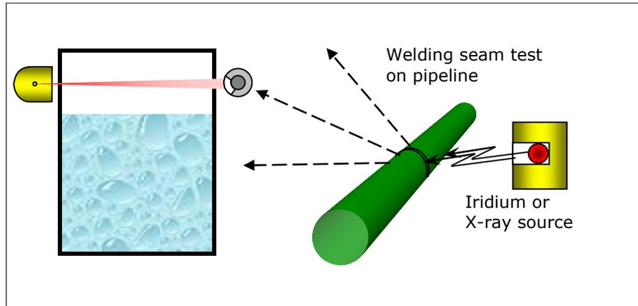
effect that interference radiation aimed at the detector (e.g. radiation emitted during welding seam tests) may trigger a false alarm or not trigger an alarm.
