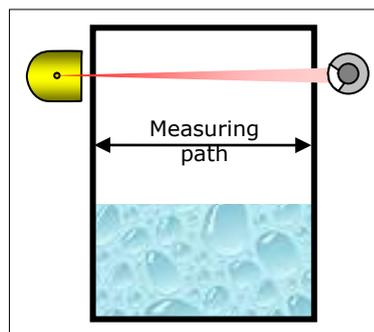
This parameter is needed only in connection with code 34 or 35. Enter here the distance covered by the radiation inside the container (in mm). Typically, this is the internal diameter of the container. If you enter "0" the function is disabled.
