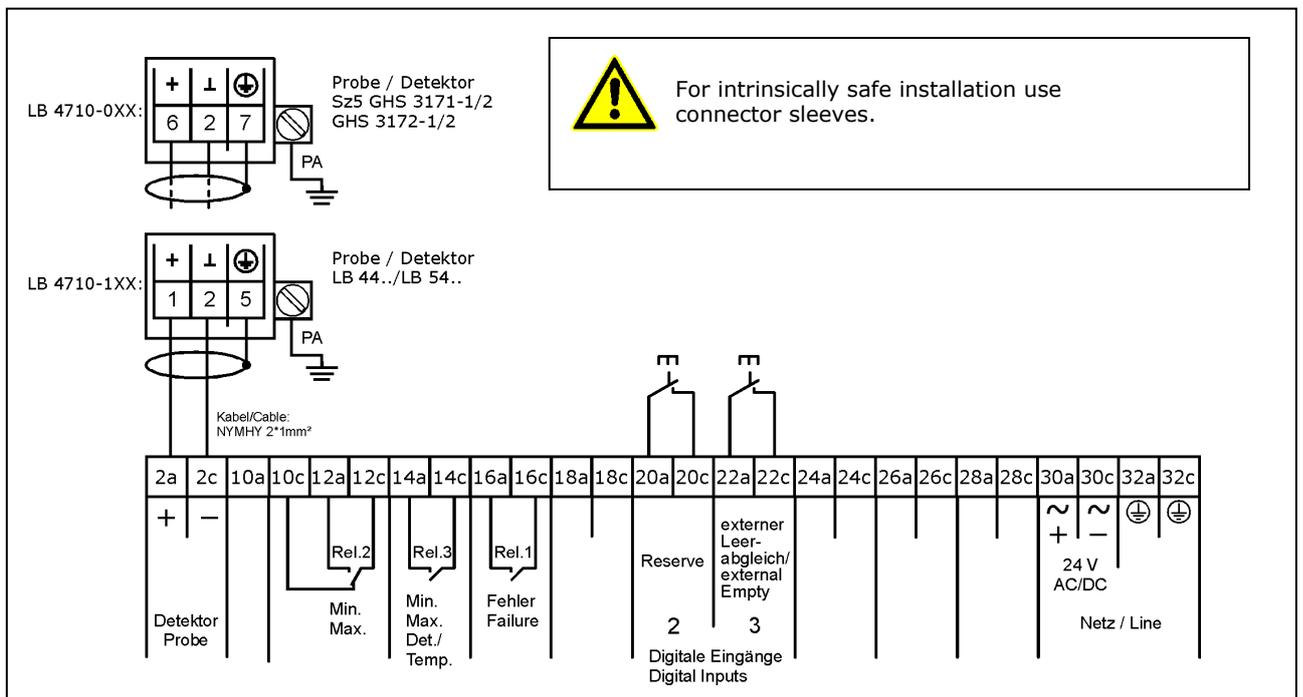
Figure 57: Connection diagram of terminal block
