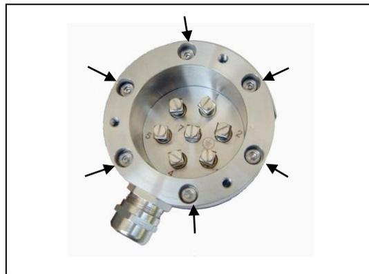
**3** Carefully pull electronic base **1** with electronics **2** and counter tube **3** out of the detector case **4**.
