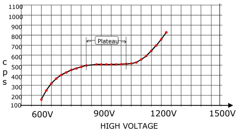
A plateau is the flat section in the characteristic curve and is typically approx. 200 V long.
