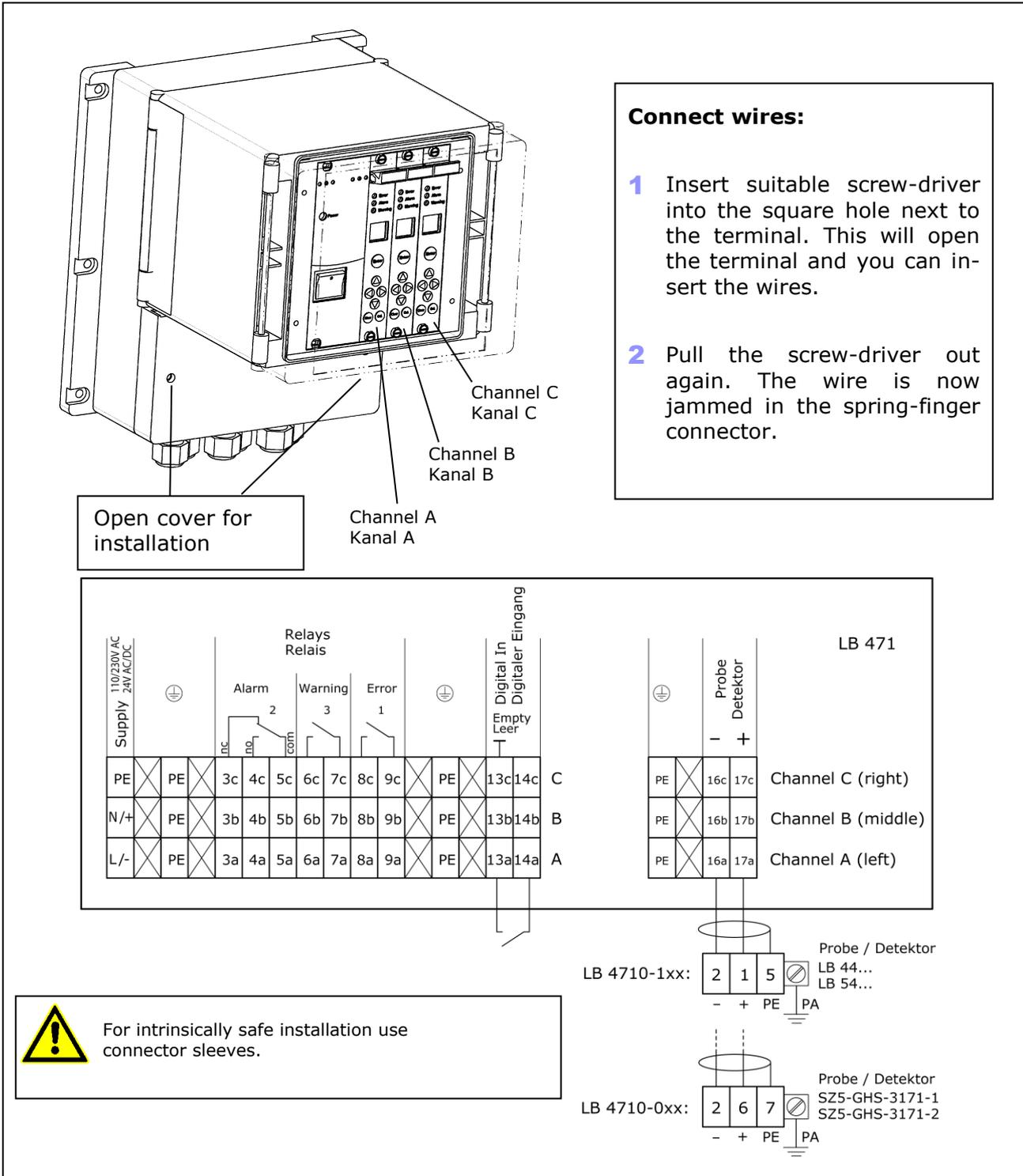
Figure 55: Connection diagram wall housing
