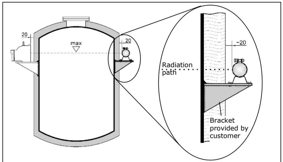
If the bracket cannot be installed on the container, then it has to be mounted on the girder located in the vicinity. Figure 10 shows three alternative proposals for installing the detector (A, B, C).
