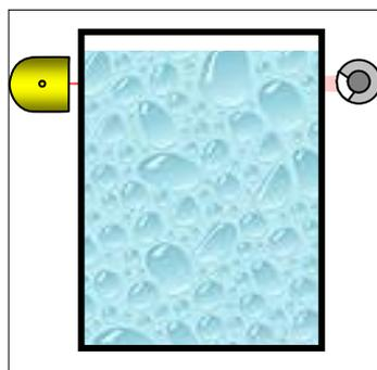
Carry out full calibration at a level above the monitoring height. Read in the count rate at this level.
