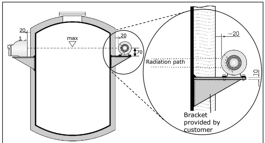
If the bracket cannot be installed on the container, then it has to be mounted on the girder located in the vicinity. Figure 15 shows three alternative proposals for installing the detector (A, B, C).
