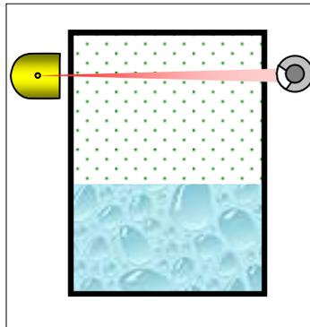
If the container is under gas pressure during operation, empty calibration also has to be carried out under this gas pressure. If this is not possible, then empty calibration may also be carried out without gas pressure, and then it has to be compensated for automatically using the entries in:
