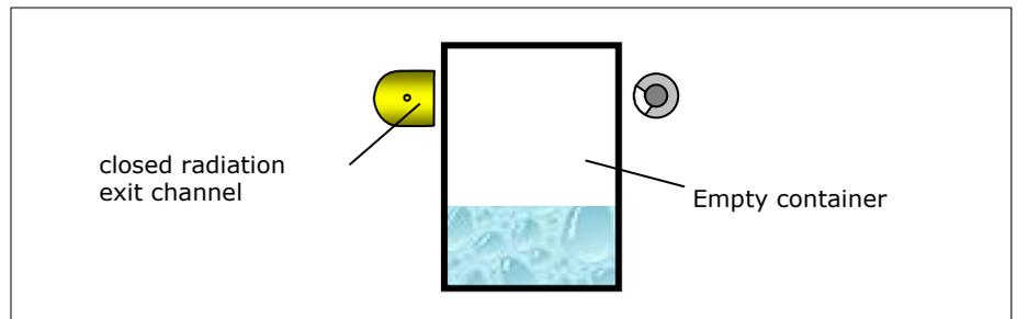
If this method is used, the detector often receives a minor amount of residual radiation from the radiation source, which is negligible for Cs-137 sources. For Co-60 sources this method may be used only if the influence of the residual radiation on the measurement can be estimated.
