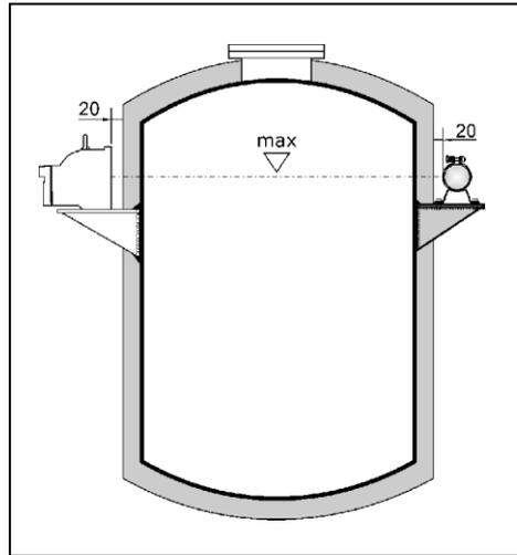
Mark the level to be monitored at the container. Position the detector there in a horizontal line with the source. At the same time, the horizontal line is the limit level where the device is switching. Make sure that the radiation window of the detector is not covered by the holder. The distance to the surface of the container or the heat insulation should be approx 20 mm.
