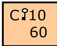
If the device is locked, all codes can be read but not edited. If the device is locked, a **key** appears on the display for all parameters.
