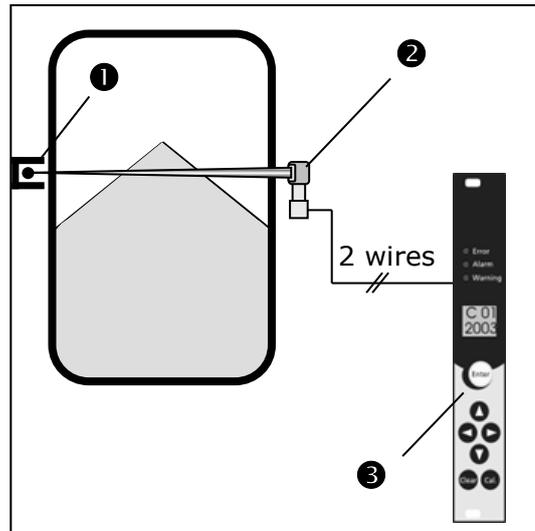
The shielded radiation source ❶ is installed outside the container on the level to be measured. A detector ❷ is installed on the opposite side of the container. The evaluation unit ❸ is connected to the detector by a 2-wire line.
