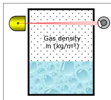
If high gas pressures are expected in the container under operating conditions and you can carry out the empty calibration only in a state without pressure, the empty count rate in code 30 has to be corrected accordingly, because the empty count rate is decreasing as the gas pressure is rising. You can carry out automatic correction with code 34. If you enter "0" the function is disabled.
