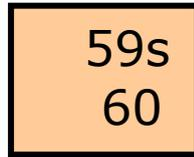
While reading in the count rate, the remaining averaging time appears on the display instead of the code number. The averaged count rate is displayed in the bottom row. You can change the start time for averaging in code 37.
