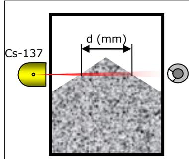
You have to enter the bulk cone diameter "d" in mm if measurements on bulk goods should trigger an alarm at a certain bulk cone diameter. Then the limit value indicates an alarm as soon as the bulk cone has reached the specified diameter "d".
