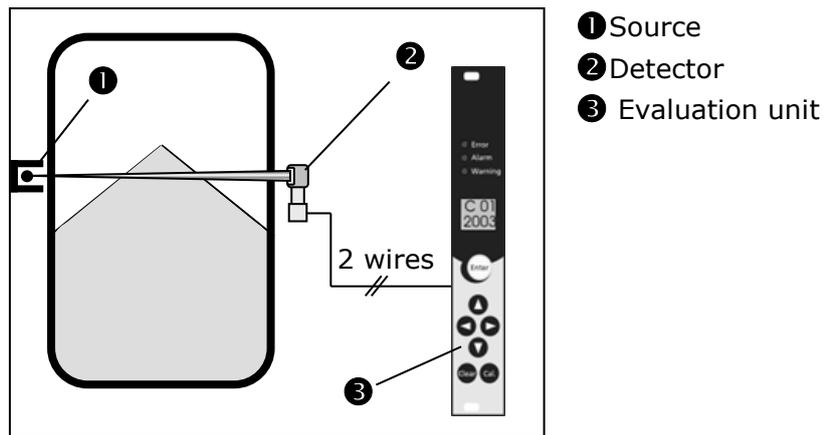
The measuring system can be employed for the detection and indication of maximum levels (overflow protection) and minimum levels (protection against dry running) and fulfills the requirements regarding:
