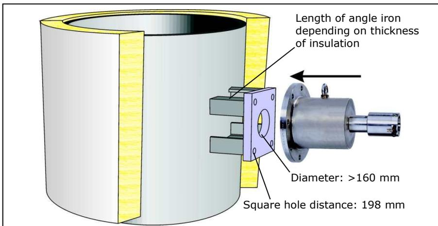
The axial radiation window, located in the center of the flange, covers the sensitive area of the detector. The radiation window must face the source.
