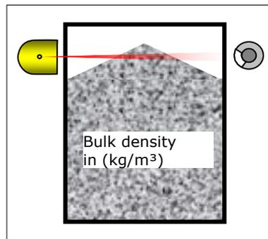
If calibration at full container is not possible, you can here enter the density of the product being measured in order to calculate the full count rate automatically. If you enter "0" the function is disabled.
