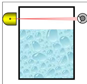
Carry out empty calibration at a level below the monitoring height. Read in the count rate at this level.
