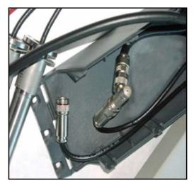
HV-divider, only a single detector is connected (see also illustration on page 100).
