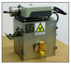
The shielding LB 7410 is supplied with the source. The source is in a shielded position. The source should remain shielded as long as the shielding is being assembled or work has to be carried out in the bunker in the vicinity of the radiation path.
