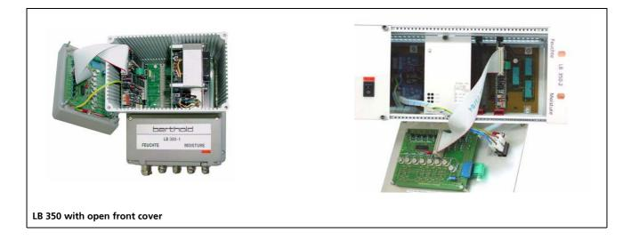
Close the jumper J4 on the CPU card LB 3940. This will set the HV control to manual voltage.
