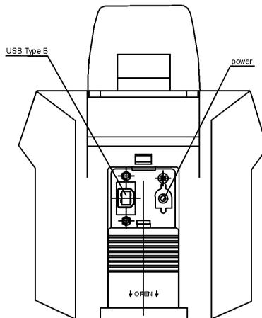
**Figure 2.4:** *Connections (rear panel of the instrument)*
