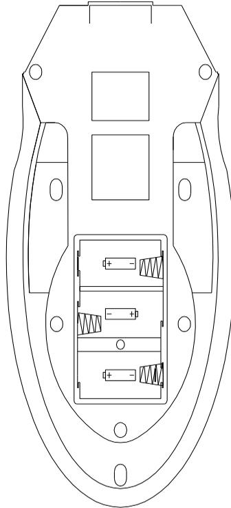
*Figure 2.5: Instrument underside with battery compartment*
