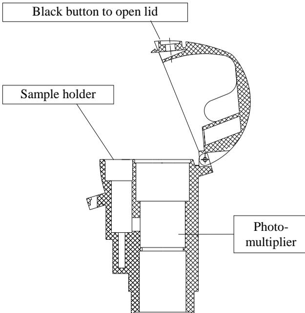
***Figure 2.3: Profile of the measuring chamber containing the sample holder and photomultiplier***
