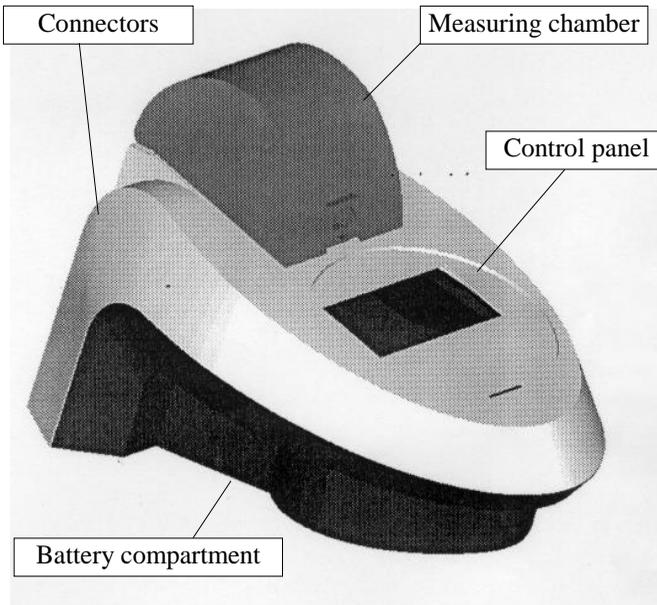
***Figure 2.1: Instrument set-up***
