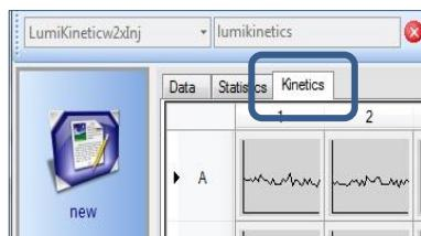
The scale of the axes can be changed by right-clicking into the curves and selecting **[Options]...**
