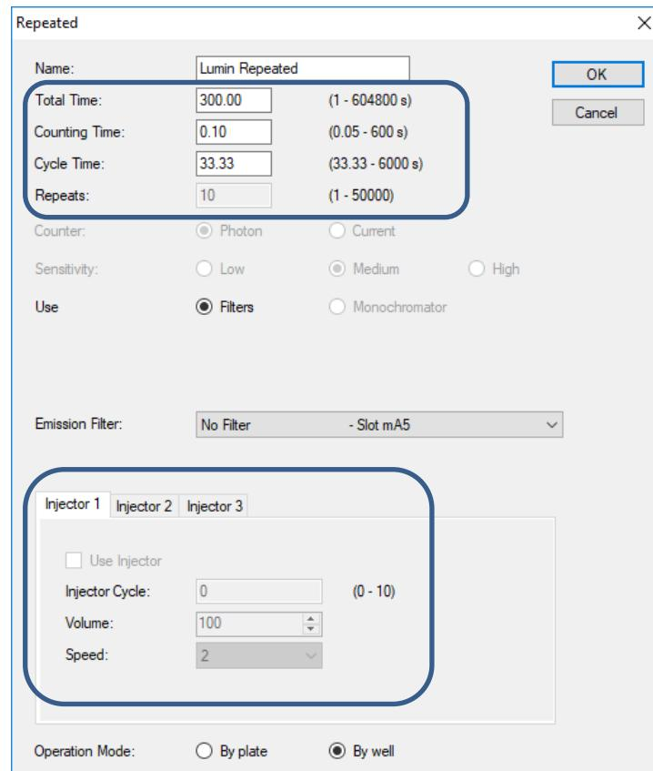
Special settings for Repeated reading are marked with a frame.
