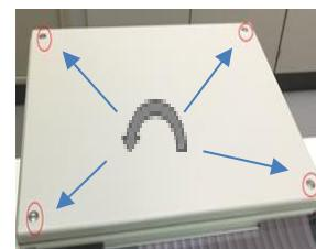
5. Remove the transportation lock indicated by the red tap. Make sure to unscrew the complete hexagonal rod attached to the horizontal support.
