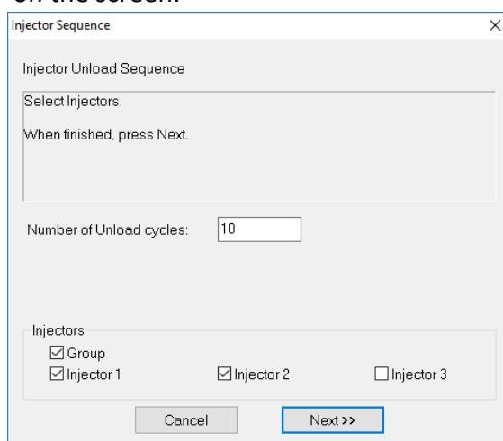
**[Number of Unload cycles]** A cycle is equivalent to the max. injection volume of the injector installed. Recommendation: 10 cycles in minimum
