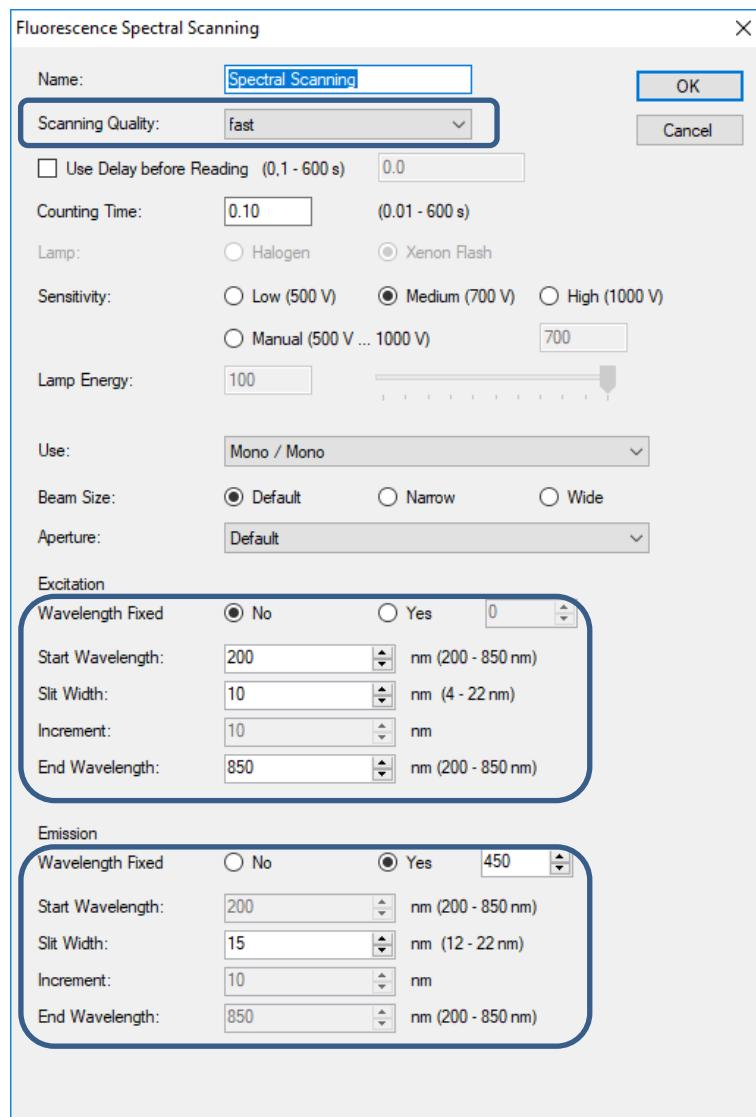
**Special settings for Spectral Scanning are marked with a frame:**
