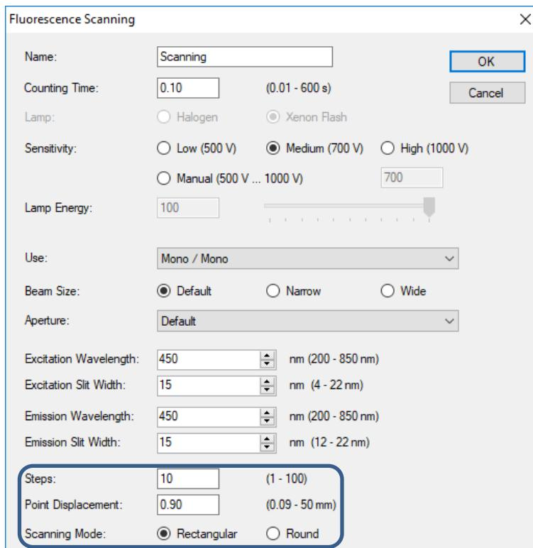
Special settings for Scanning are marked with a frame:
