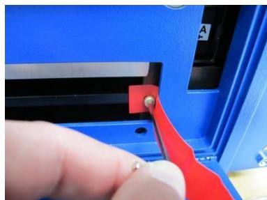
Open the big front flap and insert the transportation safety device
