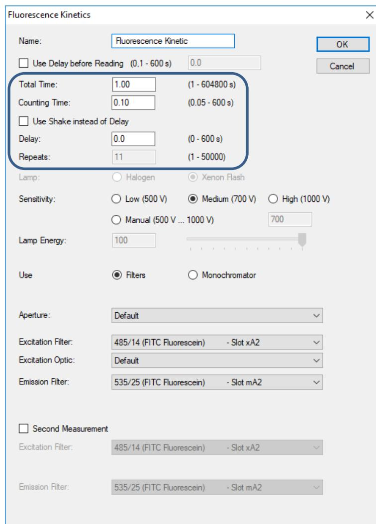
Special settings for Kinetic reading are marked with a frame.
