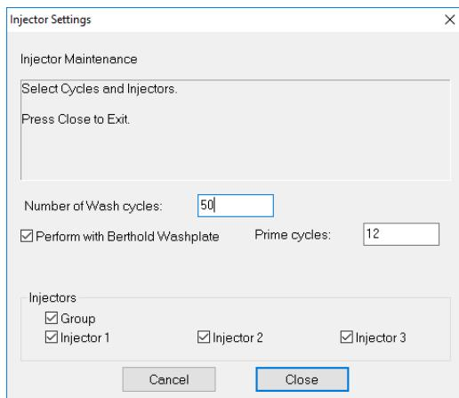
[Number of Wash cycles] usually  $\geq$  20, depending on assay reagents and microplates (see warning in section 3. below)
