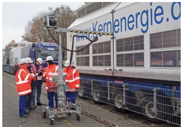
Figure 3: Neutron measurement during CASTOR transport
