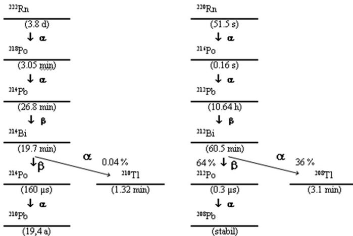
The ABPD method uses the specific measurement of the Bismuth-214 decay into Polonium-214 and the Bismuth-212 decay into Polonium-212 to compensate for natural activity.
