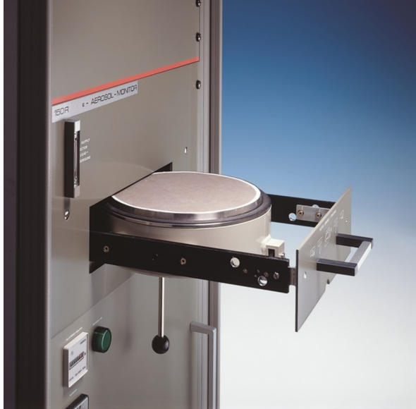
200 mm diameter filter of LB 150 D-R
