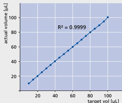
JET injectors enable the injection of liquids with an accuracy and precision better 2 %.
