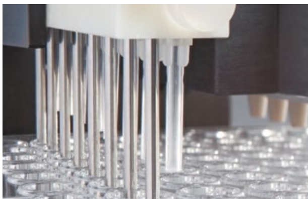
8 well parallel washer, providing consistent washing performance
