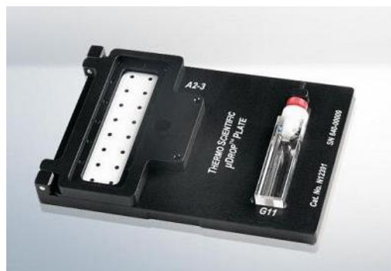
Figure 1: The \mu Drop™ plate can be used for DNA quantification using absorbance at 260 nm in a microplate reader using only 2 \mu L of sample. It also features a cuvette port for increased flexibility.
